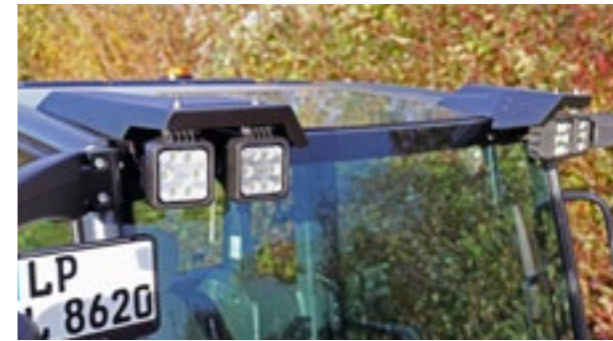
Up to four working headlights can be mounted on the front of the cabin.
